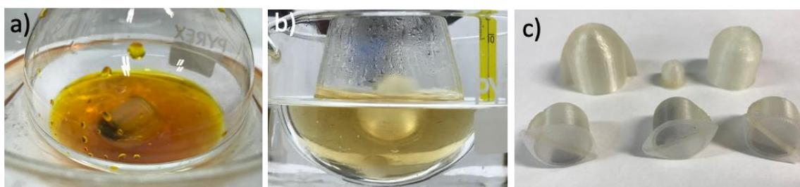
**Figure 5.** (a) Heck reaction mixture using Capsule@IRA-120-Pd(0). (b) Capsule@IRA-120-Cu(0) during CuAAC. (c) Different shapes and sizes of 3D-printed capsule prototypes.
