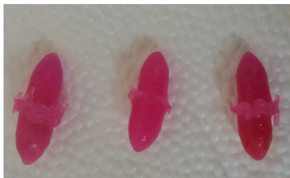
Figure S2 Dil-C (Fluorescent dye encapsulated capsules). a) Alginate capsules with Dil-C dye. b) Alginate-MMT capsules with Dil-C dye. The Capsules with MMT looks intact compared to one without MMT.
