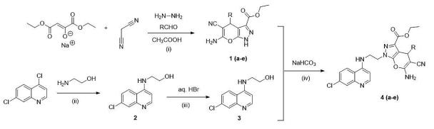
**Figure 7.** Reagents and conditions: (i) EtOH, reflux 1–2 h, *R* = benzaldehyde, 4-ethylbenzaldehyde, isobutyraldehyde, 4-hydroxybenzaldehyde and furaldehyde; (ii) reflux 1h; (iii) reflux 3 h and (iv) DMSO, r.t.
