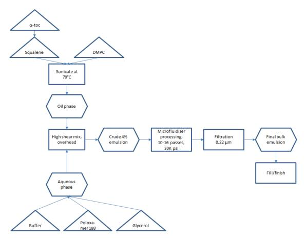
**Figure 1.** Small-scale (≤1 L) process flow diagram for production of SE.
