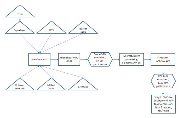
Figure 6. Large-scale (200 L) process flow diagram for one-pot production of SE.
