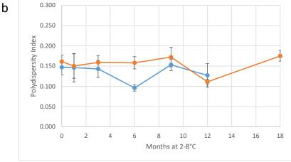
**Figure 5.** Physical stability of the two large-scale batches from Table 7 when stored at 2–8  $^{\circ}$ C. Droplet diameter (a) and polydispersity index (b) remain stable for a minimum of 12–18 months. Error bars represent the standard deviation of 8–9 measurements.
