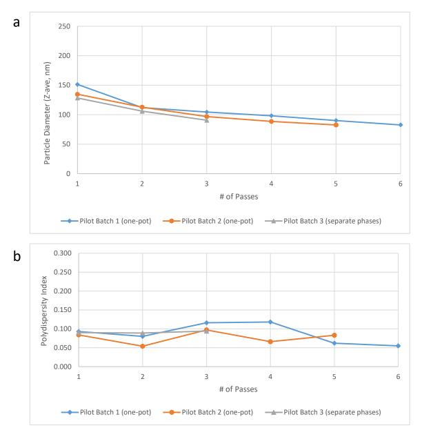
**Figure 3.** Droplet diameter (a) and polydispersity index (b) as a function of number of passes through the Microfluidizer processor in  $30\% \ v/v$  oil-in-water emulsion batches produced at the pilot scale (10 L) using the one-pot approach or the traditional separate phases approach as indicated.
