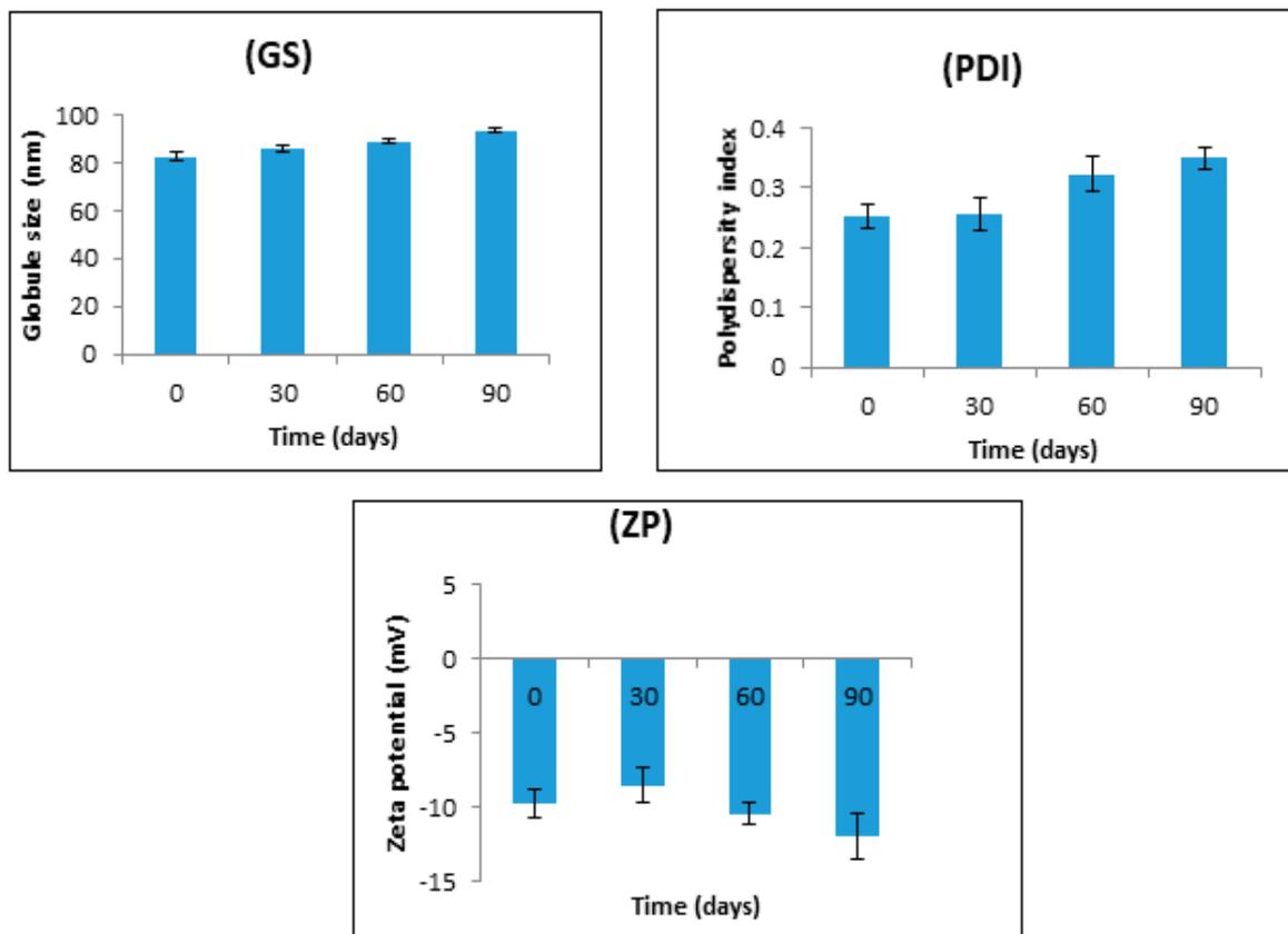
Figure 8. Effect of storage for up to three months at  $40 \pm 2$  °C and  $75 \pm 5\%$  RH on the globule size (GS), polydispersity index (PDI), and zeta potential (ZP). The data are presented as the mean  $\pm$  SD,  $n = 3$ . The slight increase in particle size, PDI, and ZP was not significant ( $p > 0.05$ ) for adjacent sampling points.
