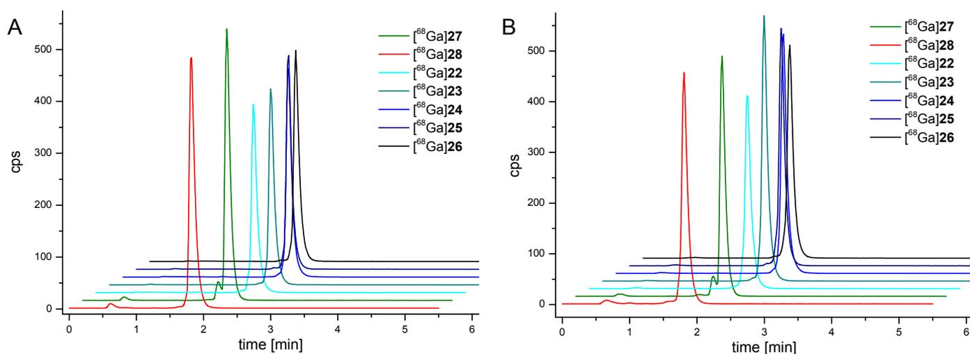
Fig. S1: Typical analytical radio-HPLC chromatograms of  $[^{68}\text{Ga}]\mathbf{22}$  –  $[^{68}\text{Ga}]\mathbf{26}$ ,  $[^{68}\text{Ga}]\mathbf{27}$  and  $[^{68}\text{Ga}]\mathbf{28}$  directly after  $^{68}\text{Ga}$ -radiolabeling (A) and after 90 minutes incubation with human serum at  $37^\circ\text{C}$  (B).
