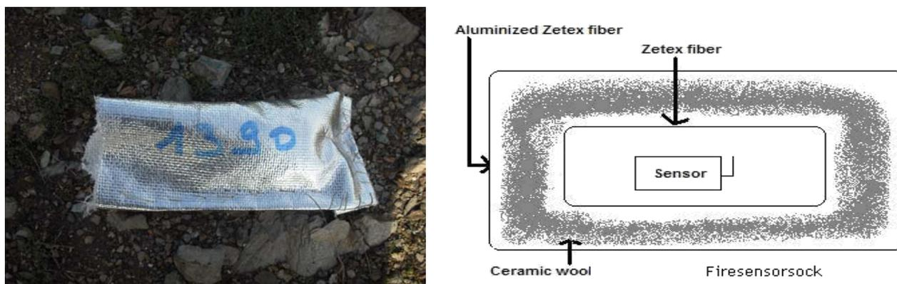
The Firesensorsock consists in several layers of thermal insulation materials: a layer of simple Zetex fiber, a layer of ceramic wool and a final layer of aluminized Zetex fiber. These layers are fixed to one another with Kevlar thread. We thus achieve a level of protection allowing the sensor to support a prolonged fire contact and also wireless communications without any disturbance.
