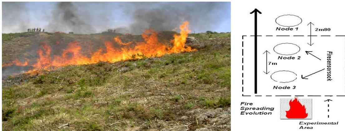
**Figure 4.** MICA 3<sup>rd</sup> GEN Experimental Area with 12 sensors on a square with 2 m 50 in width and 2 m distance between the nodes.
