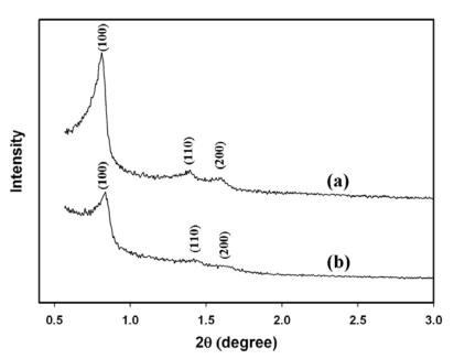
Figure 1. XRD pattern of (a) SBA-15 and (b) SBA-15(HRP).
