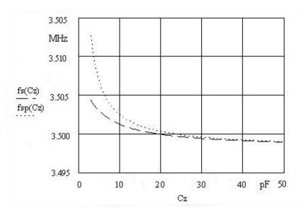
Figure 2. Quartz crystal pulling sensitivity from 3 to 50 pF.
