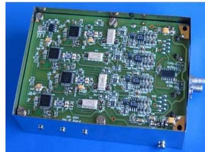
A switch follows the antenna and commutes between the antenna signal (SA) and the correlated noise (SCN) (Fig. 3) from a controlled noise source (CNS), used for calibration purposes. A CNS has been designed to provide three temperature points (300, 400 and 500 K), so as to perform two types of calibration: internal hardware calibration and absolute radiometric calibration.
