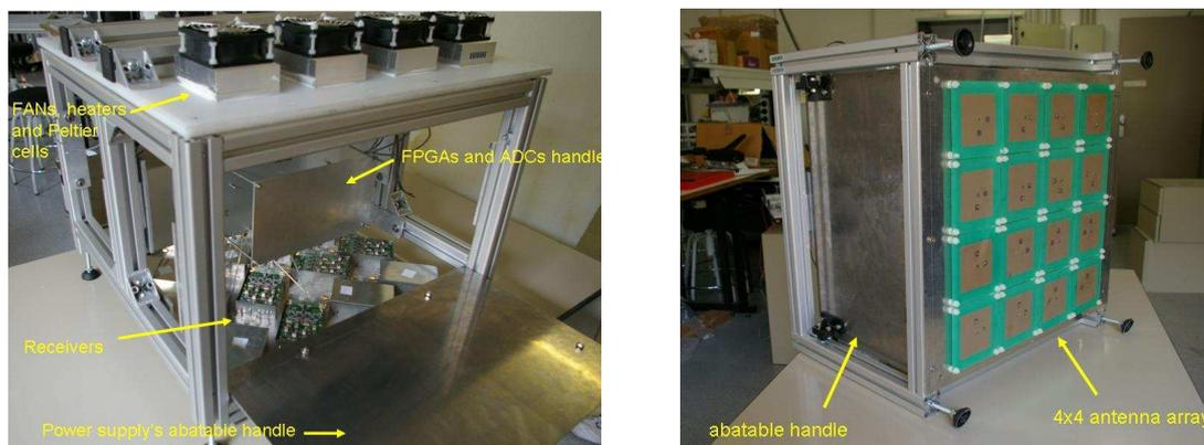
PAU-RAD is a full polarimetric radiometer, so that the delivered results are the four Stokes parameters (eqn. 1). The Stokes parameters fully characterize the polarization state of partially polarized thermal radiation. This polarized thermal radiation is related to different phenomena such as the angle incidence, the sea surface salinity (SSS), the sea surface temperature (SST), the sea surface roughness (SSR), wind direction, foam...
