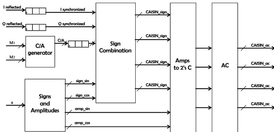
**Figure 3.** Detail of the main cores that compose the DDM generator: (a) ‘Sign and amplitudes’ block in Fig. 2 and (b) ‘Oscillator block’ in Fig. 3a.
