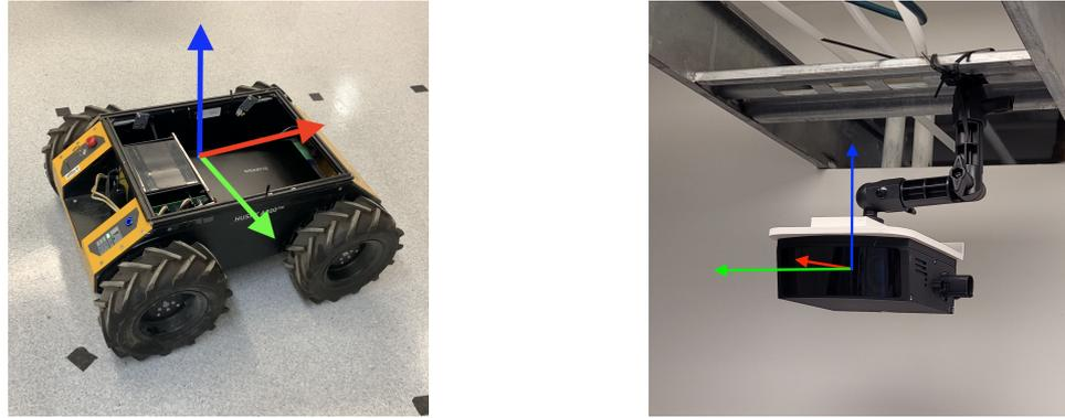
**Figure 1.** Experimental setup for evaluation of the LiDAR-based distributed state observer: unmanned ground vehicle (UGV) setup (left), and solid-state LiDAR used for remote sensing (right).
