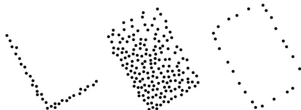
**Figure 2.** The  $xy$ -projection of the UGV robot's clustered point cloud in real time for  $z_s \leq z_r$  (left), for  $z_s > z_r$  (center), and the convex hull of the cluster  $xy$ -projection (right).
