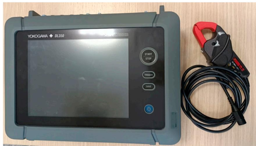
**Figure 13.** Data acquisition system used to measure current signals in the IM2.
