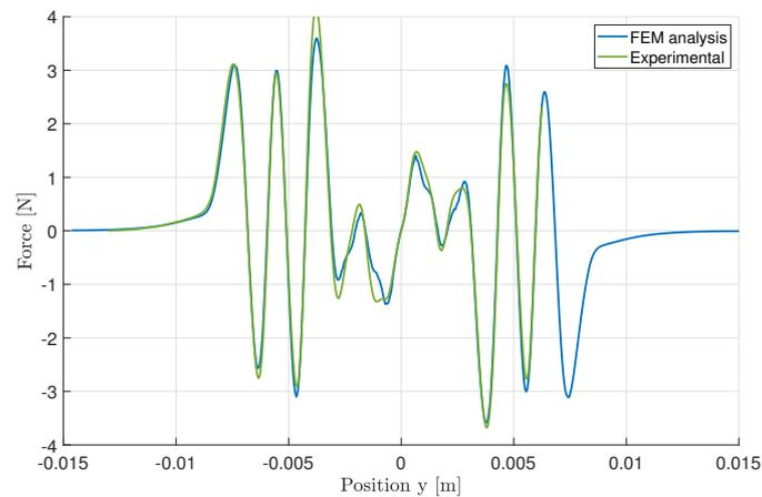
**Figure 7.** Magnetic force along the vertical axis ( $z$  direction) between the head-to-head magnet tower and the ferromagnetic core. This plot shows the finite element analysis (FEA) processed on the measured geometry including the imprecisions due to machining.
