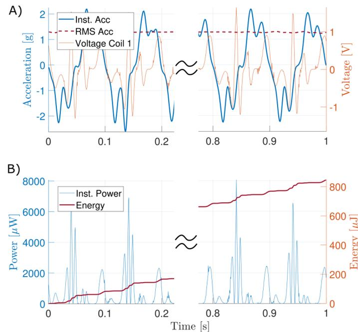
**Figure 9.** (A) Voltage measured across a  $25 \Omega$  load connected on a single coil for an external excitation at 10 Hz and with an amplitude of 8 mm. (B) Power and energy harvested on a single coil by the inertial EMEH.
