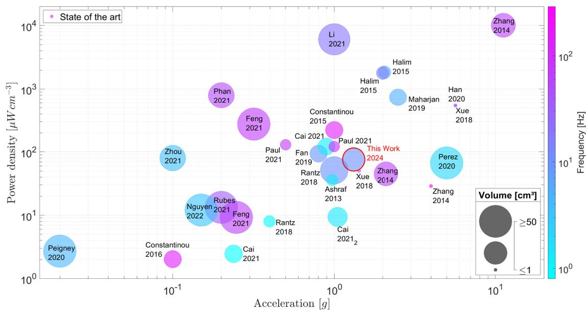
**Figure 2.** Comparison chart gathering on the same footage various inertial EMEH experimentally tested in the literature [3,23–42]. The power densities, accelerations, frequencies of operation and volumes of EMEHs are depicted on the same figure in order to highlight the dependencies related to those parameters. The red circle identifies the proposed EH discussed in this work.
