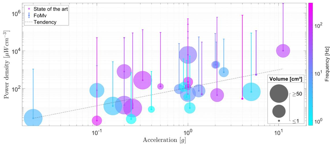
**Figure 3.** Performances of selected inertial EMEH and the distance from their idealized power densities (based on FoMv). The power densities, accelerations, frequencies of operation, and volumes of EMEHs are depicted in the same figure in order to highlight the dependencies related to those parameters. Their attached bar represents the distance from their idealized yield.
