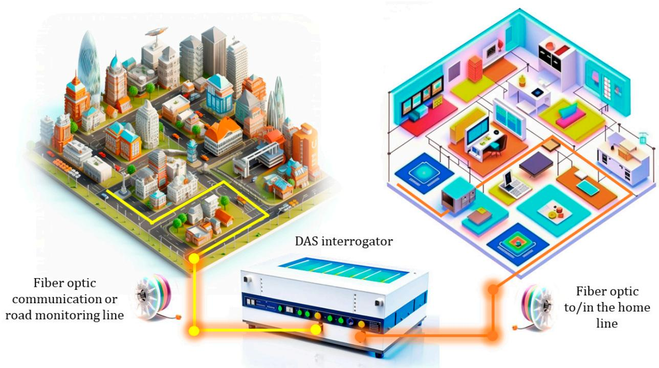
**Figure 1.** Scheme of DAS interrogation for a smart city (left) and smart home (right).
