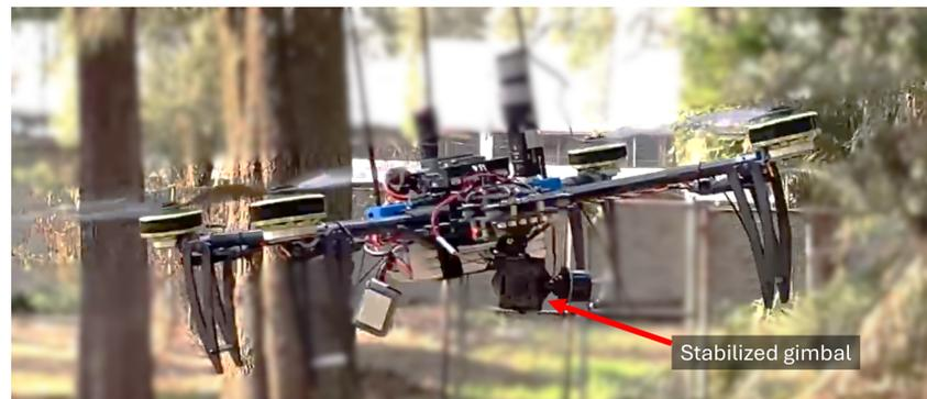
**Figure 8.** Stabilized gimbal in hover flight test with external perturbations.
