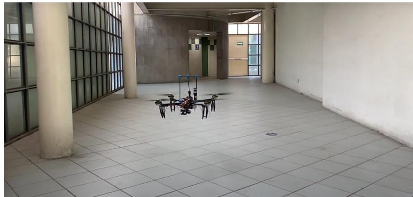
**Figure 9.** Indoor flight tracking control test with stabilized optical flow.
