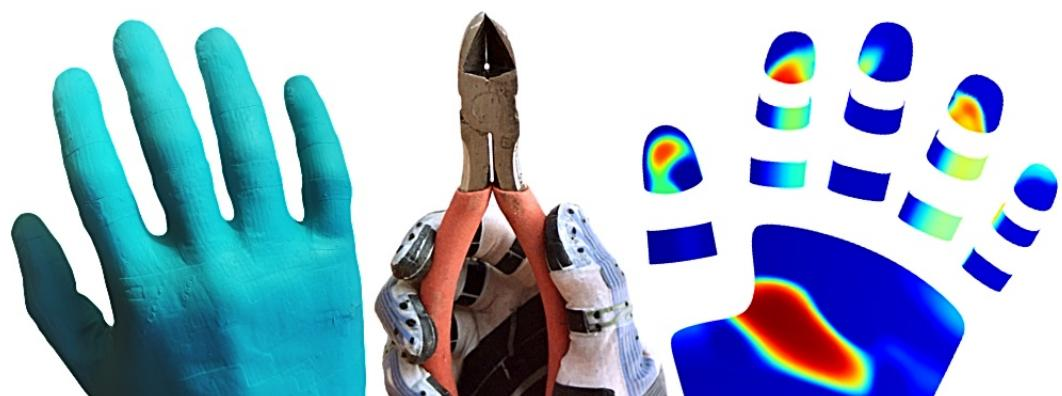
**Figure 1.** We create thin and elastic sensor gloves from elastic rubber-like materials (left, center) to capture tactile data (right, highest forces in red) during dexterous manipulation and tool use (center).
