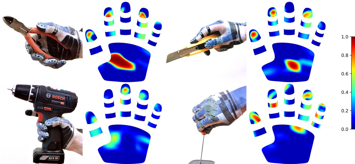
**Figure 14.** Manipulation experiments with a sensor glove prototype and corresponding tactile sensor readings. Sensor readings are visualized with a colormap (right) and a CAD model of the glove.
