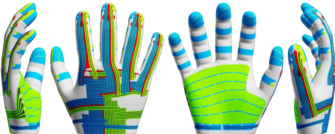
**Figure 2.** CAD model of our sensor glove. Electrodes for sensor rows and columns are shown in green and blue, spacing constraints in black, and ground electrodes in red.
