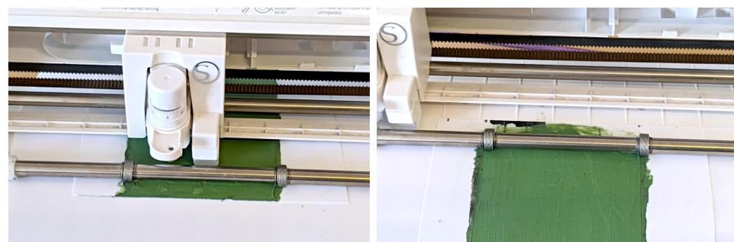
**Figure 5.** Cutting electrically conductive silicone traces.
