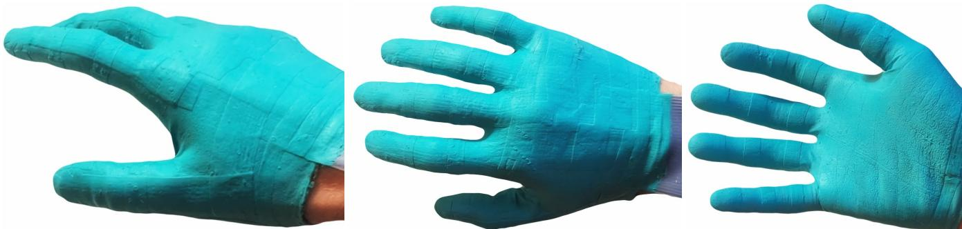
**Figure 12.** Fully assembled and painted sensor glove on a human hand.
