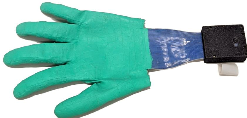
**Figure 9.** Fully assembled and painted sensor glove with readout module.
