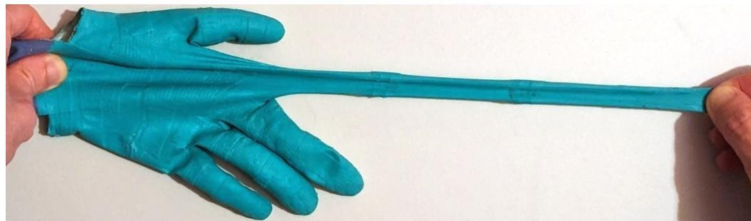
**Figure 19.** Our sensor glove is completely made from highly elastic rubber-like materials.
