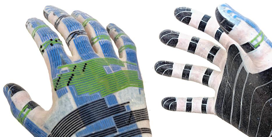
**Figure 8.** Partially finished sensor glove on a human hand, with sensor elements and conductor bundles transferred to the glove surface. A subset of conductive traces is colored in green and blue for easier identification.
