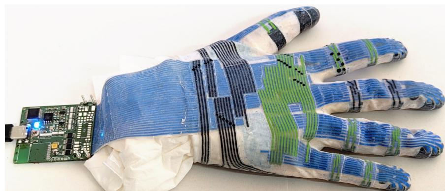
**Figure 7.** We join conductors on different layers in a partially finished sensor glove by stuffing the glove and punching vertical vias with a conductive silicone-covered needle. Silicone films for a subset of conductors are painted prior to cutting and transfer for easier identification.
