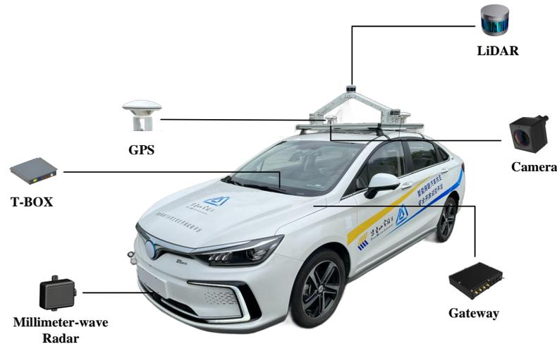
Figure 10. Experimental vehicle platform.
