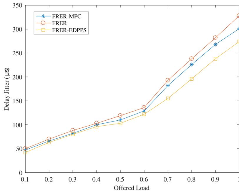
**Figure 7.** Performance of delay jitter under different offered loads.
