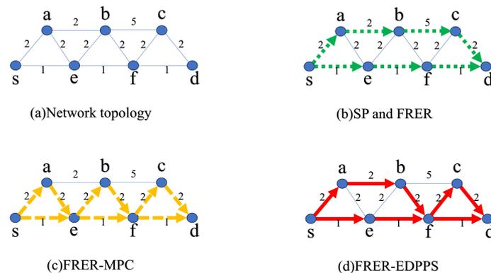
**Figure 3.** A working example of FRER-EDPPS.
