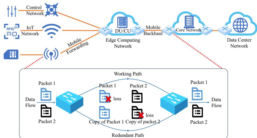
**Figure 1.** Illustration of FRER mechanism in edge computing network.
