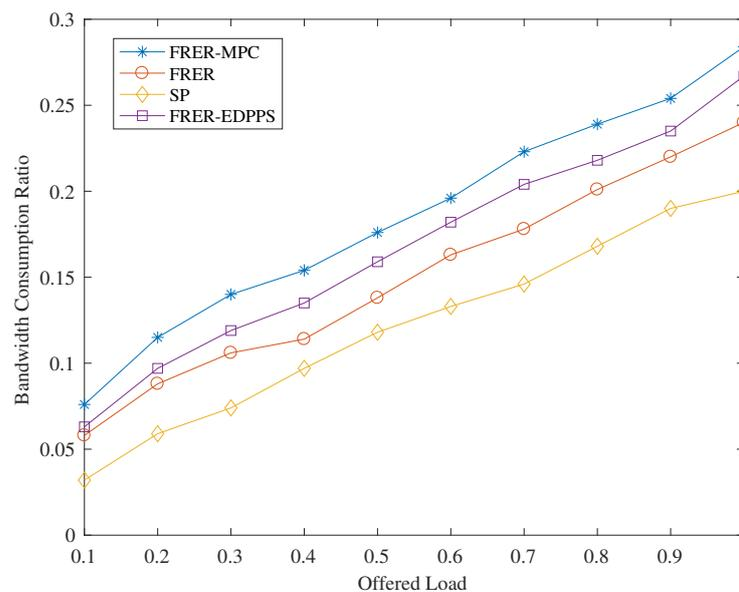
**Figure 6.** Performance of bandwidth consumption rate under different offered loads.
