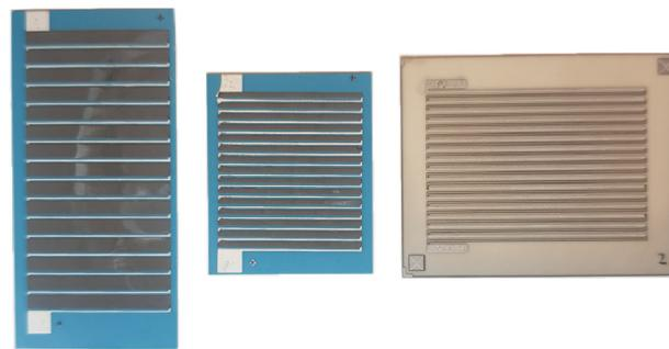
**Figure 2.** Examples of planar  $\mu$ TEGs.
