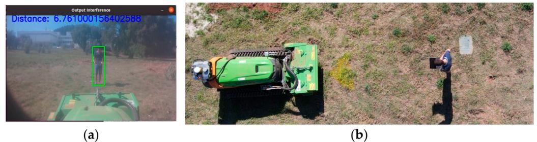
**Figure 9.** Test to verify the measurement from the camera. (a) Procedure for one of the stages of testing the vision system algorithm in the field. (b) The person located 6 m from the front camera of the Sentry.
