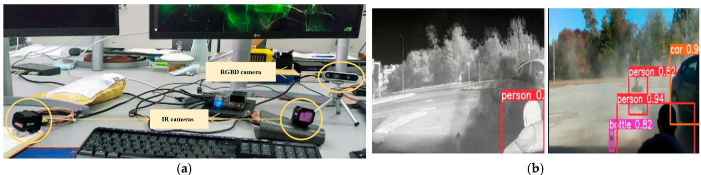
**Figure 7.** Test to verify the operation of YOLOv5. (a) Setup with two thermal cameras, one RGB camera, and one depth camera; (b) YOLOv5 response.
