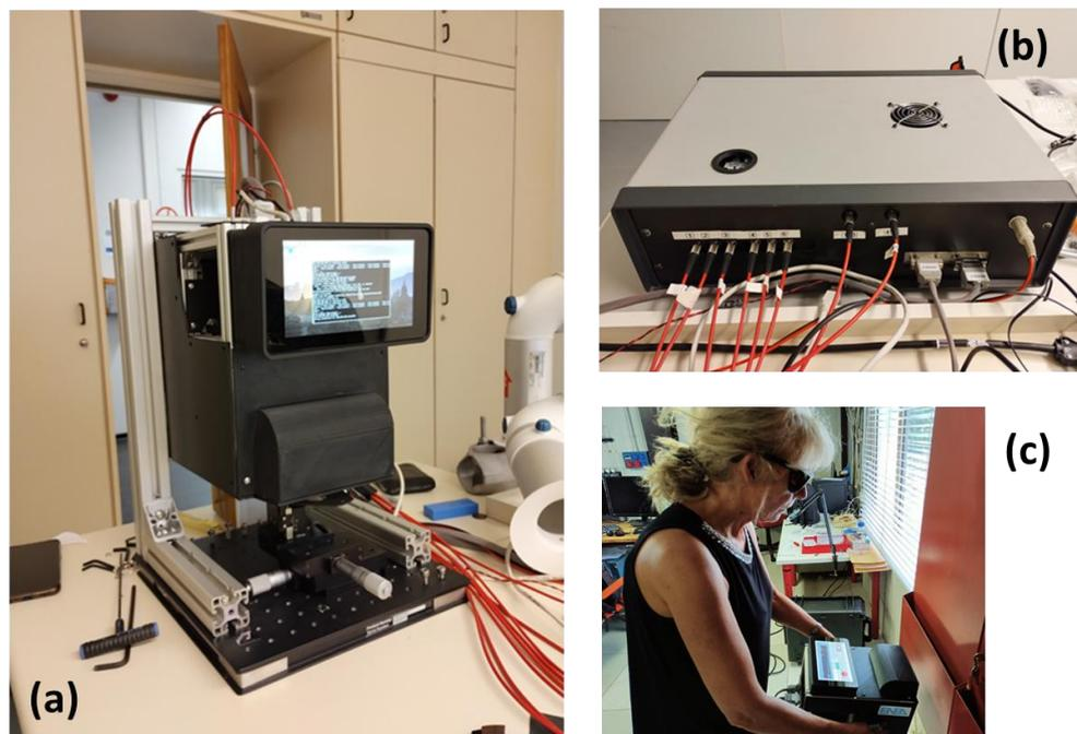
**Figure 1.** (a) LIBS sensor head mounted on a structure for static measurements; (b) the instrument box; (c) sensor head operated in a handheld mode.
