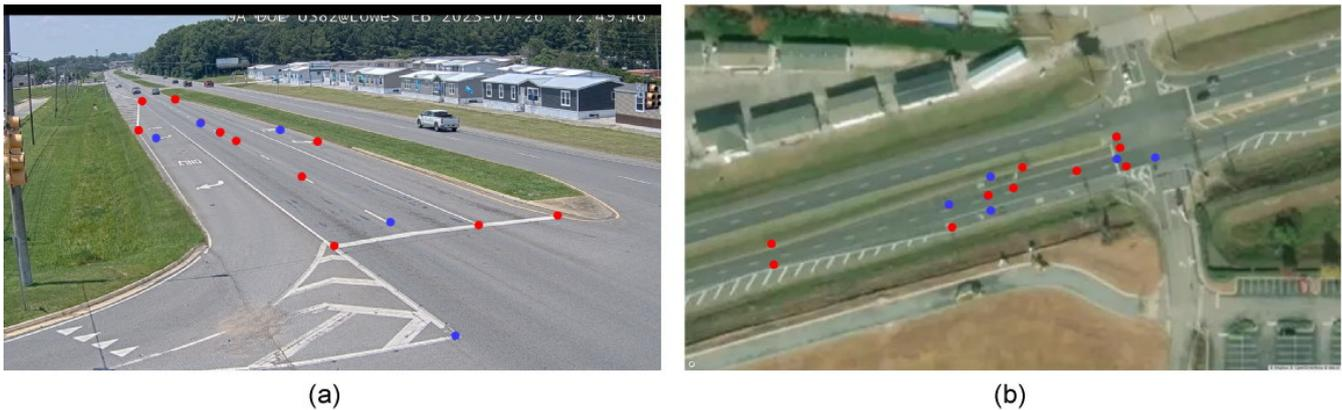
**Figure 6.** Data points collected by a single roadside camera for camera calibration. The red dots are used for the transformation matrix calculation, while the blue dots are used for validation purposes. (a) Data points shown on an image plane. (b) The corresponding data points on a Google Map.
