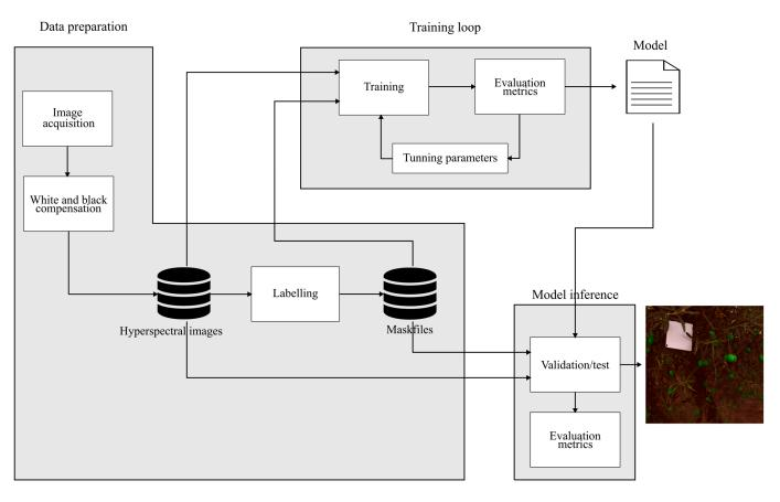
**Figure 1.** Framework of the proposed model for the identification of the Gordal green olive variety in hyperspectral images.
