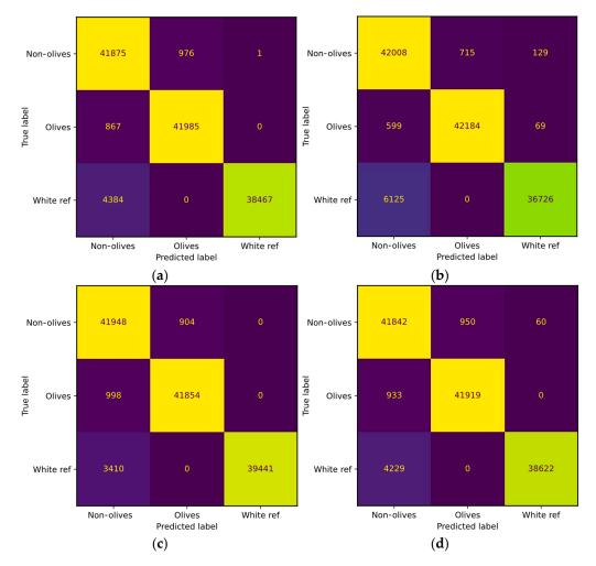
**Figure 2.** Confusion matrix with the validation dataset. (a) LR classifier with the Bandnorm technique. (b) LR model without normalization. (c) SVM model with the Bandnorm technique. (d) SVM model without normalization.
