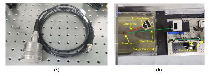
ultrasonic waves. The ultrasonic waves are picked up by the hydrophone and used as an input signal for the experiment.
