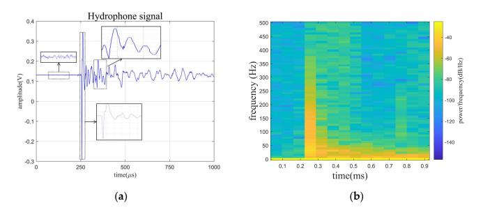
**Figure 10.** The time-domain signal received by the hydrophone and the spectrogram of signal. (a) Time-domain signal. (b) The spectrogram of signal.
