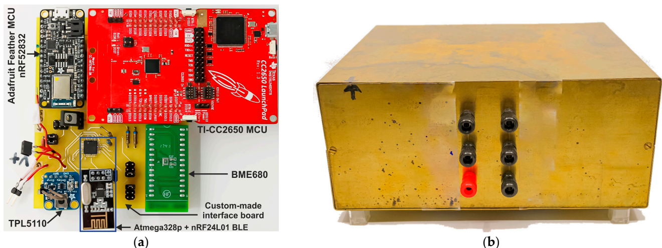
Figure 7. Overview of the test board used to connect different MCU platforms where only the tested MCU is connected during the characterization (a), and the designed shielding box used during the experimental test to omit RF disturbance from external environment (b).
