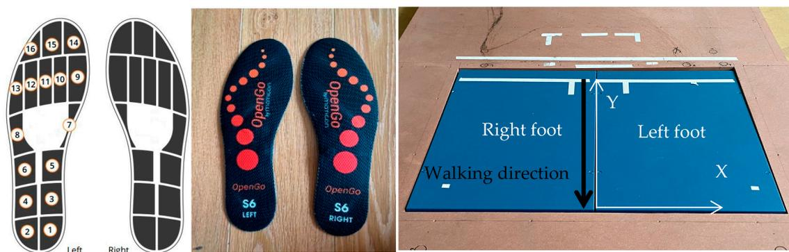
**Figure 2.** Experimental equipment. **Left:** layout of the pressure sensors of Moticon insoles. **Middle:** Moticon insoles. **Right:** AMTI force plates.
