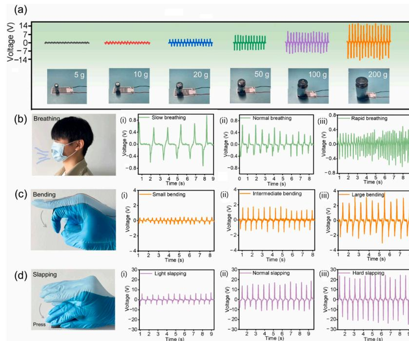
**Figure 14.** The characteristic output signal of the sensor: (a) under different weight pressure; (b) breathing at different frequencies; (c) bending fingers at different angles; (d) slapping at different strengths. Reprinted with permission from [144]. Copyright 2023 Elsevier Ltd.
