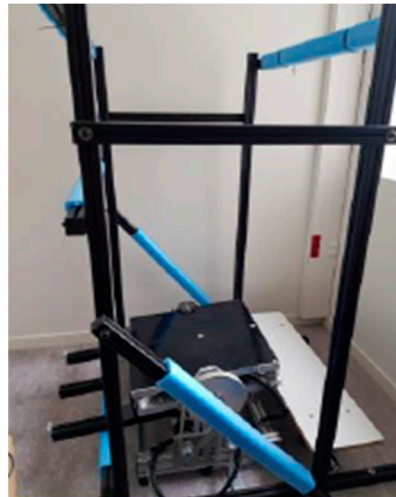
Figure 1. The force platform used in the experimental setup, surrounded by its foam-clad aluminum frame. This platform could be tilted in the AP axis or held stationary horizontally.
