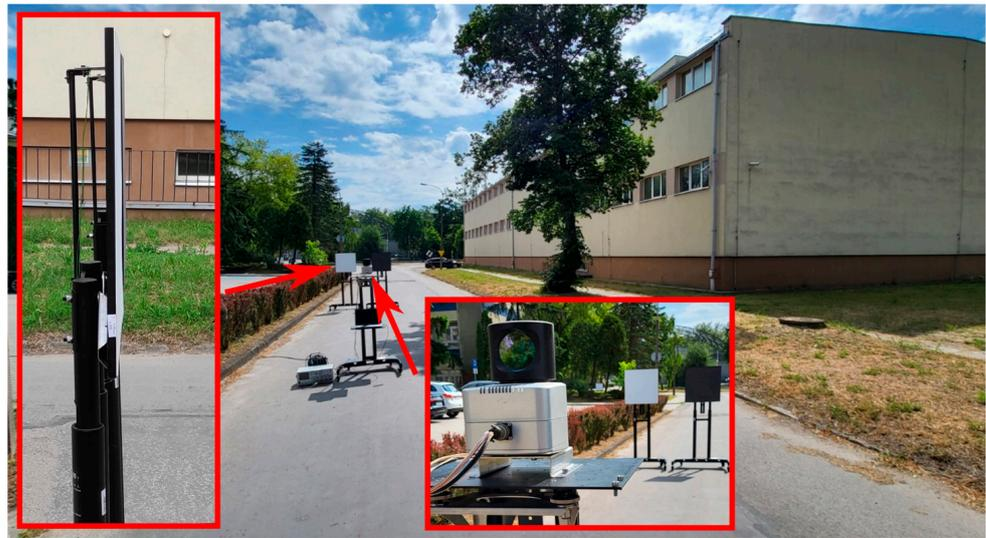
**Figure 8.** Photo of the field test site showing the scanner and reference targets.
