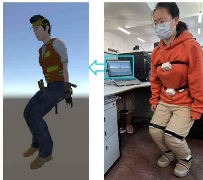
Figure 4. Real-time human body and digital human model.
