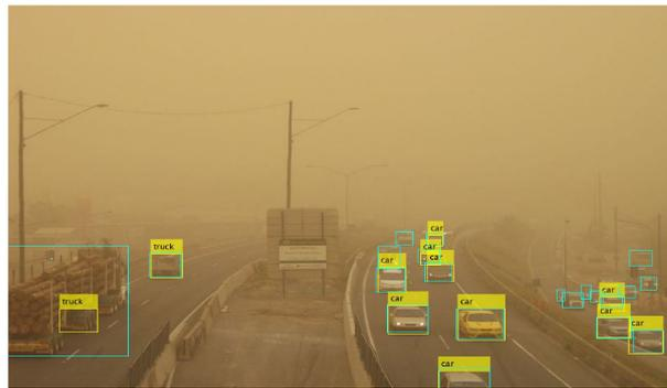
**Figure 13.** Wrong detections from YOLOx in a sandstorm.
