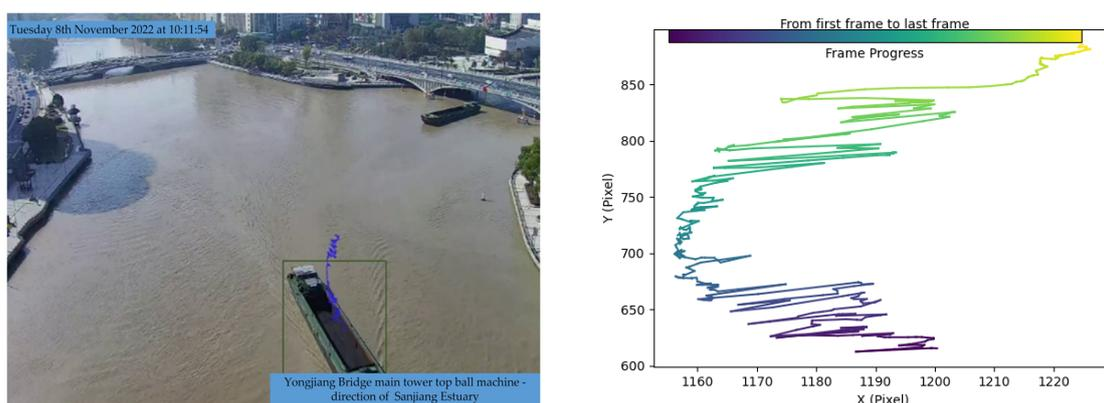
**Figure 13.** Obtaining vessel trajectories based on bounding boxes
