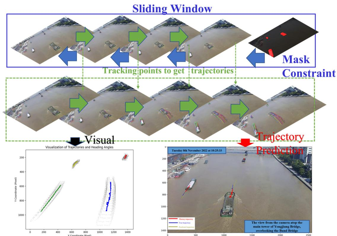
**Figure 4.** Technique for the acquisition and prediction of vessel trajectories.
