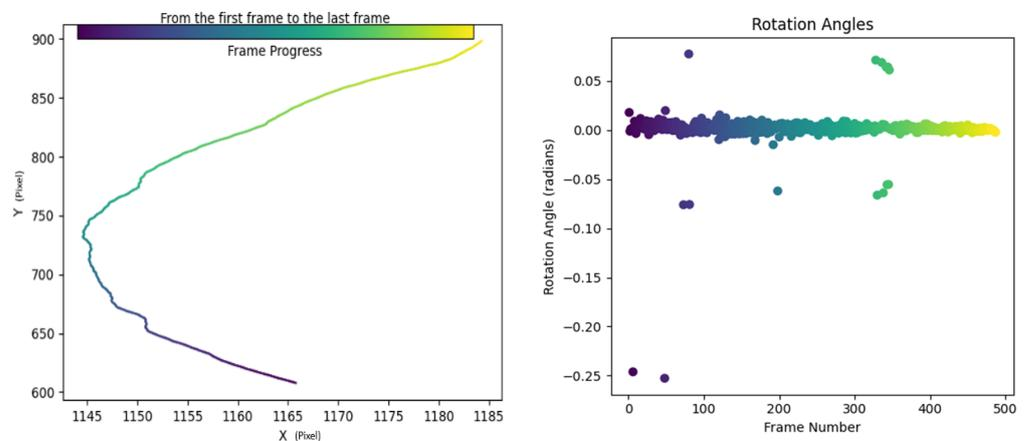
Figure 16. Long-term vessel trajectories and heading angles.
