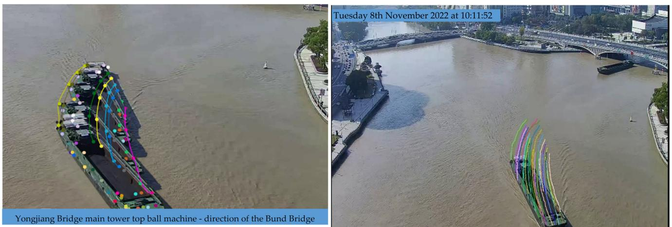
Figure 15. Multi-feature point cluster tracking method.
