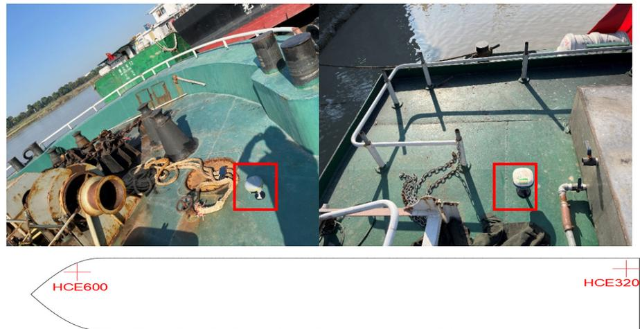
Figure 8. Experimental ship GPS equipment layout.
