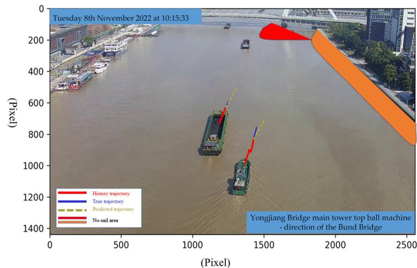
**Figure 17.** Predictive and alert illustration diagram.
