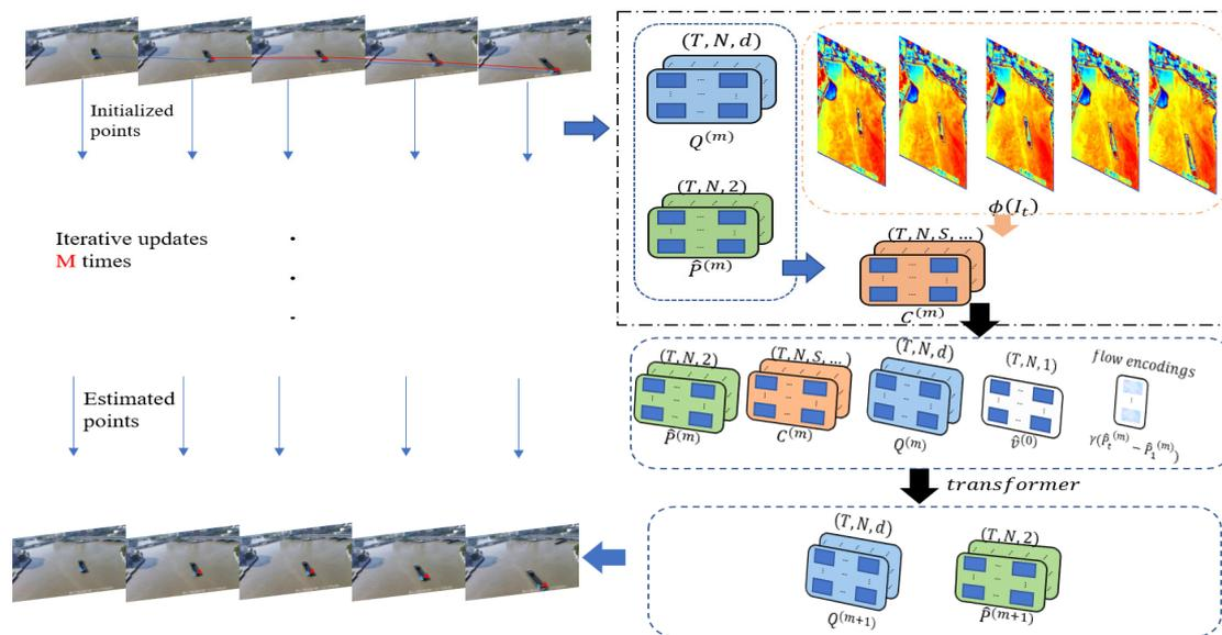
**Figure 2.** The framework for tracking the motion trajectories of multiple feature points.
