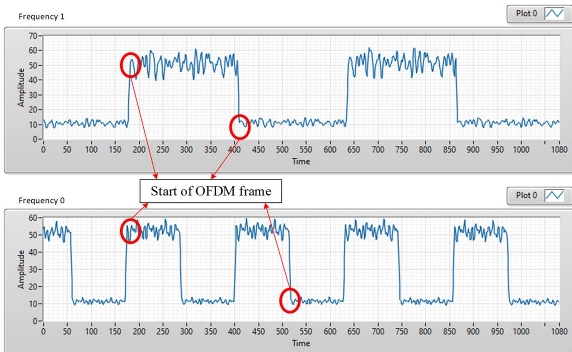
**Figure 11.** Received signals by the USB camera FL3-U3-132C-CS (PointGrey rolling-shutter camera).
