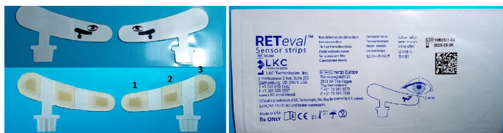
Figure 5. The RETeval sensor strip. The strip contains three electrodes: (1) the active-positive, (2) the reference-negative, and (3) the ground electrode in a single adhesive tape. The image on the right provides the information label of the sensor strips used in the present study.
