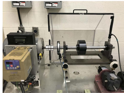
Figure 12. Experiment setup for the bearing inner race fault [35].
