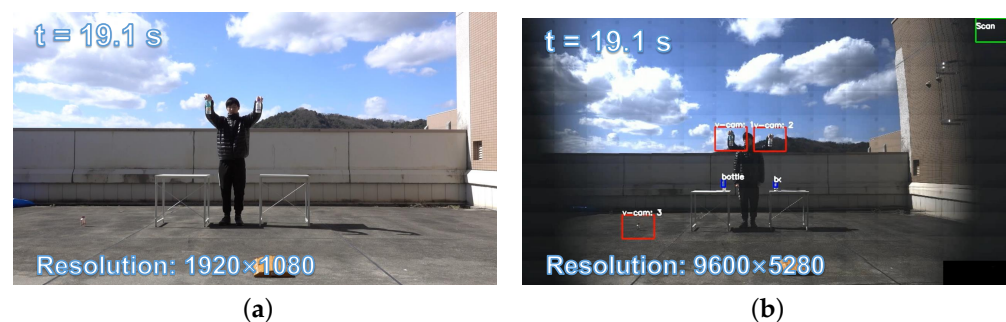
Figure 10. The 1920 \times 1080 input images from the digital camera and panoramic stitched 9600 \times 5280 images from the PTZ camera: (a) input image of digital camera and (b) panoramic stitched image from the PTZ camera.
