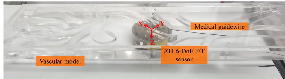
**Figure 7.** The configuration of the 6-DoF F/T sensor to acquire the contact forces generated from the interaction between intravascular tools and the vasculature.
