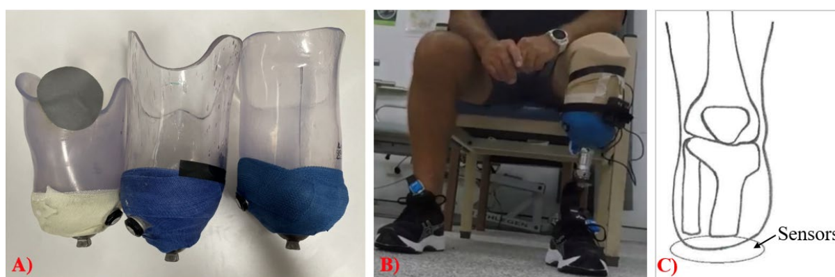
Figure 7. Experimental setup: (A) participants' check sockets, (B) participant wearing the sensor system, (C) sensor placement on the distal end of a residual limb, where one SingleTact and one Loadpad force sensor were placed.
