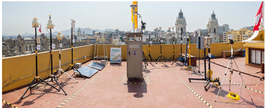
Figure 1. Place of the data collection campaign and the arrangement of the sensors. The reference station (Teledyne) is located in the center.
