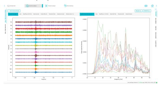
**Figure 17.** Time and frequency custom data visualizations. On the left side, the signal is filtered from 5 to 45 Hz, and on the right side, the spectrum of the channels is visualized within a bandwidth ranging from 1 to 100 Hz.
