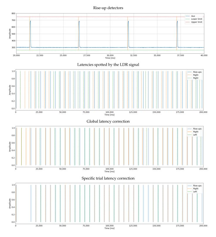
**Figure 15.** Automatic marker synchronization results. The top figure shows the signal generated by the LDR. The second figure visualizes the latencies in the system. The third figure shows what happens when all latencies are corrected with the same adjustment value, and the final plot has adjusted the latencies individually for each marker.
