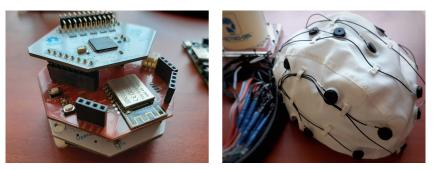
**Figure 1.** The OpenBCI system is equipped with a Daisy extension board and a WiFi shield for up to 16 channel support and 8 k SPS. It also includes an EEG cap with conductive gel for improved conductivity.
