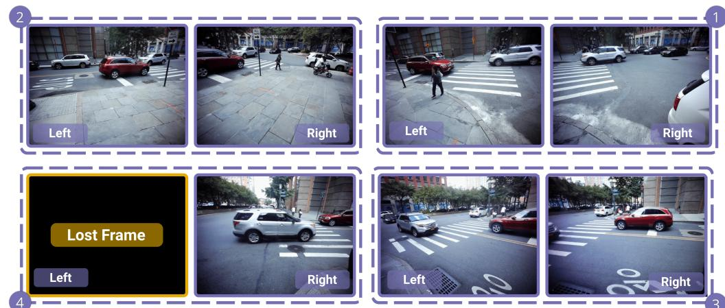
**Figure 10.** Mosaic rendering of the synchronized frames from recording session one at the Chase Center intersection that can be played as a video. Four sensors with two cameras each (numbered in the corners) provide eight different views for comprehensive analysis of the intersection. If a camera did not successfully record during a particular frame, its block is turned black, such as the left camera of sensor 4 in this example.
