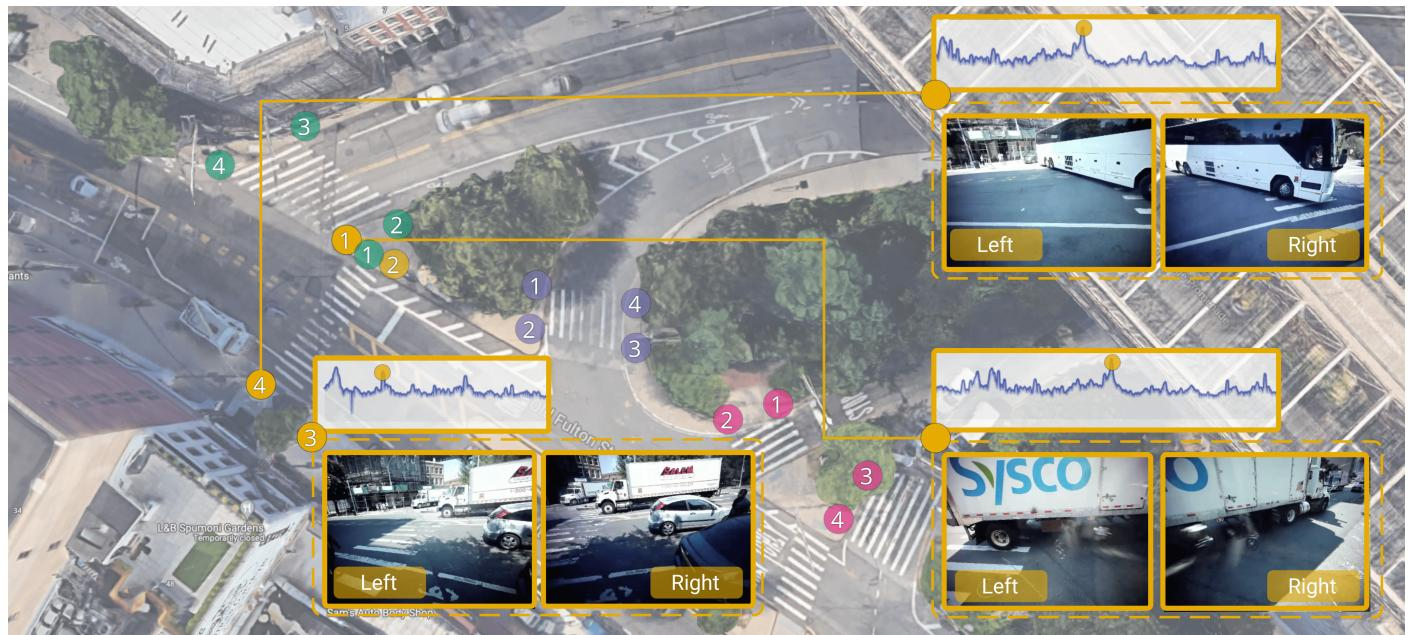
**Figure 12.** Sensor positions during data acquisition at DUMBO, Brooklyn. Colors indicate recording sessions and numbers denote the sensor. Above each synchronized video frame, we highlight the relative data point in the audio time series (in decibels). It can be shown that events that can be seen in the video, such as the passing of a bus, have a corresponding peak in the audio data.
