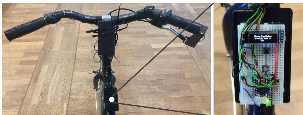
Figure A5. Cyclist's point of view with the installed sensors and the hidden control box.
