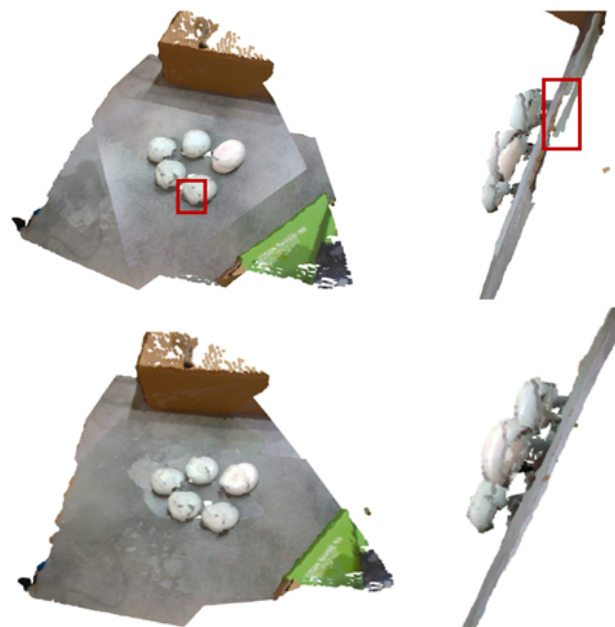
Figure 6. upper row: Examples of the initial alignment using the camera parameters, bottom row: Examples of the finer alignment of the developed method. Red boxes point out misalignments.
