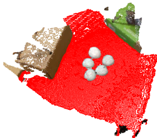
Figure 5. Plane segmentation; points belonging to the detected ground plane are visualized with red color.
