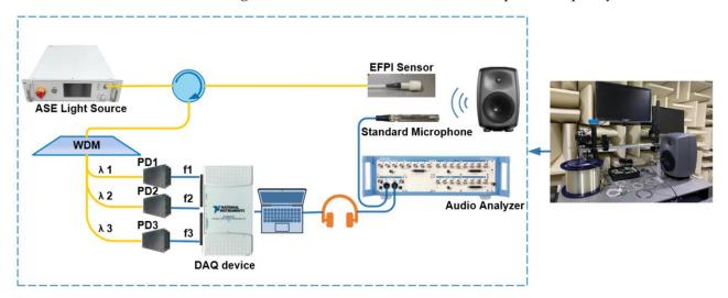
Figure 1. Schematic of the three-wavelength EFPI acoustic sensor system.
