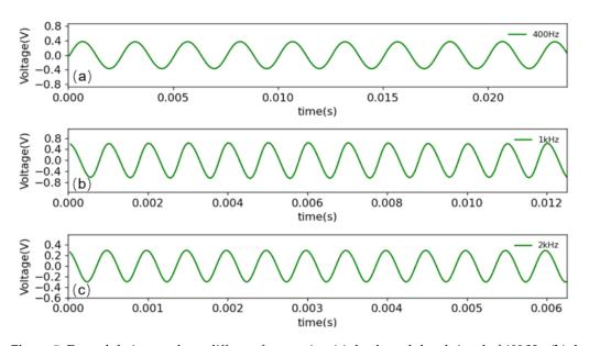
**Figure 5.** Demodulation results at different frequencies: (**a**) the demodulated signal of 400 Hz, (**b**) the demodulated signal of 1 KHz, (**c**) the demodulated signal of 2 KHz.
