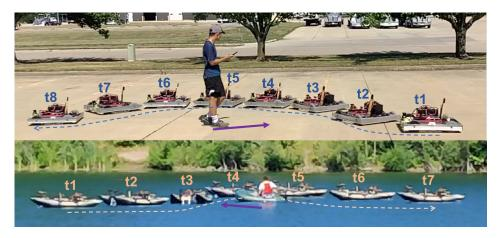
**Figure 1.** Motion lapse images of a UGV and a USV avoiding a dynamic obstacle using the same trained DRL agent. The trajectories of the vehicles are shown as dashed lines. The direction of the instantaneous velocity of the obstacles is shown as purple arrows.
