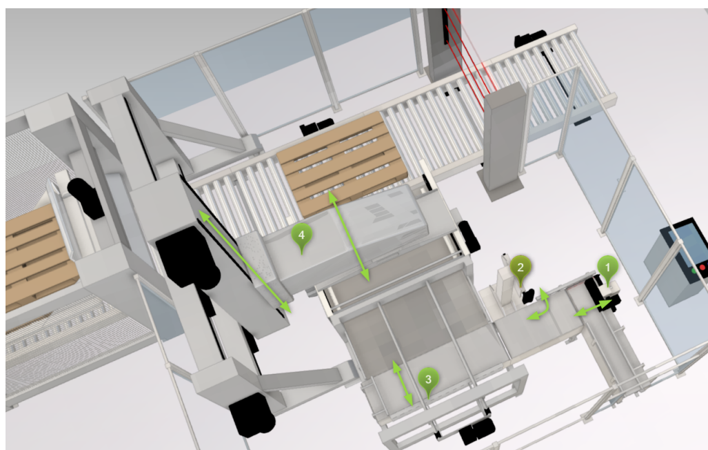
Figure 9. Simulation model used for evaluation: end-of-line palletizing portal packaging system. Motion controlled by PLC applications are marked in green. Physical control units: Nr. 1 pusher, Nr. 2 rotary vane, and Nr. 3 carriage. Virtualized control unit: Nr. 4 gripper arm.
