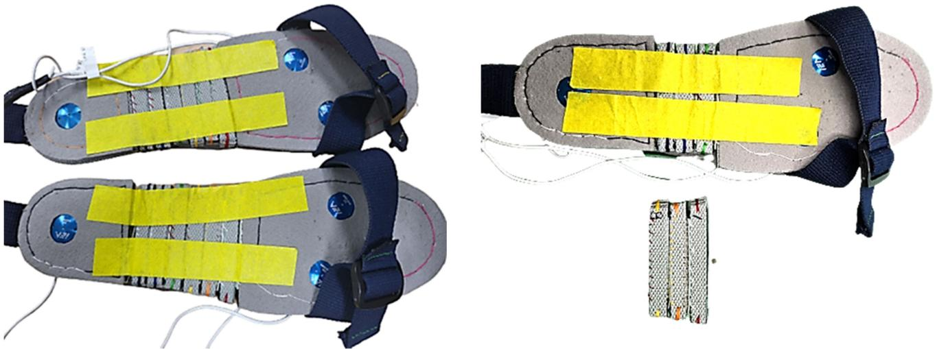
**Figure 1.** Developed shoes with three uniaxial load cells. By removing the middle blocks, the overall shoe size can be adjusted to precisely position the sensor on the subject's heel and their 1st and 5th metatarsal. One block is approximately 10 mm wide.
