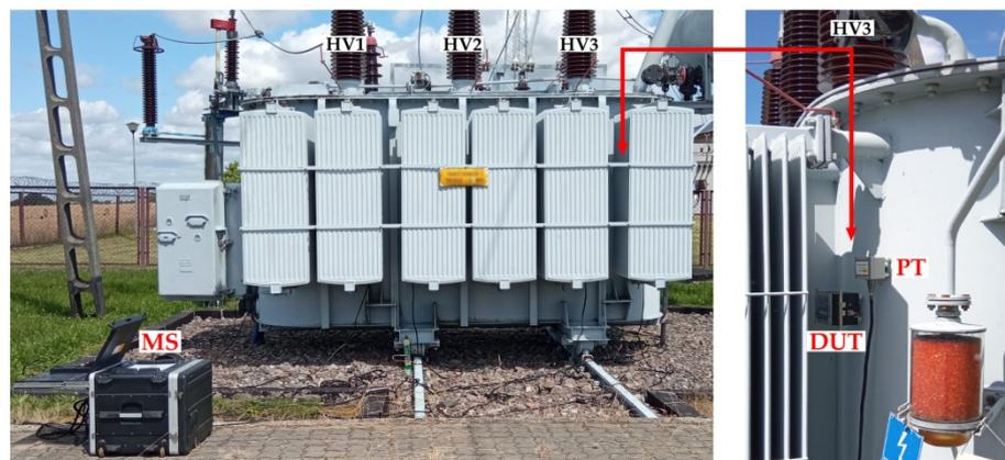
**Figure 13.** Monitoring of partial discharges in the HV3 phase of a 10 MVA power transformer: MS—reference monitoring system PDtracker Portable; PT—piezoelectric transducer of the reference monitoring system; DUT—tested low-cost PD monitoring system.
