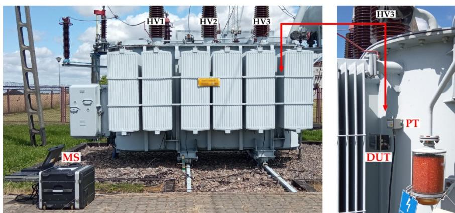
**Figure 13.** Monitoring of partial discharges in the HV3 phase of a 10 MVA power transformer: MS—reference monitoring system PDtracker Portable; PT—piezoelectric transducer of the reference monitoring system; DUT—tested low-cost PD monitoring system.
