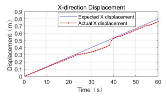
Figure 11. Comparison of expected and actual displacement in the X-direction of base truss crawling.
